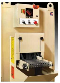
The IL-885 conveyor includes variable speed controls and adjustable parts guides to handle a wide range of blasting applications.
