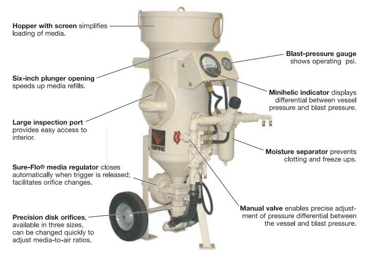
Empire SafeStrip<sup>™</sup> portables are designed specifically to handle fine, light media used in the cleaning and stripping of delicate substrates. SafeStrip portables quickly and safely remove old coatings, dirt, oil, corrosion and other unwanted residues from soft metals, rubber, plastics and other sensitive surfaces. They are ideal for work on statues, monuments, machinery and molds, and in many other applications requiring a "light touch."
